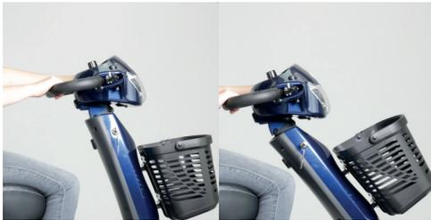
**Photo 2** Upright tiller position      **Photo 3** Angled tiller position
