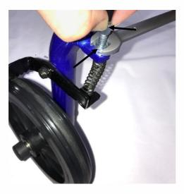
Hold the top of the cable gland (arrowed) with your fingertips or a pair of pliers.
