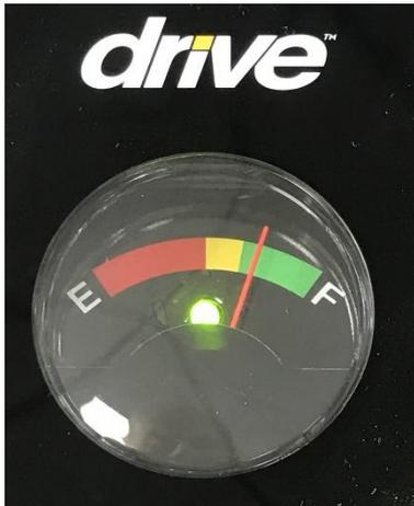
The needle in the battery gauge on the scooter tiller will show the following battery power:
