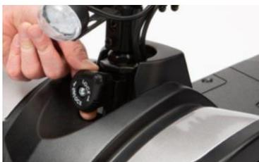
6. Lock front tiller by pulling the locking knob out and turning 90°.
