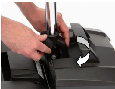
4. Turn the handle to release the battery pack, then lift out the battery pack from the main body of the scooter.
