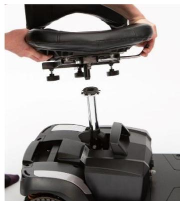
5. Replace the seat and rotate it until it locks in to its correct position.
