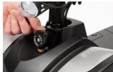
2. Unlock front tiller by pulling the locking knob out and turning 90°.
