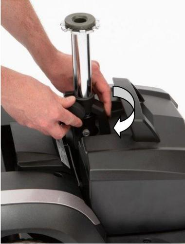
2. Turn the handle to release the battery pack, then lift out the battery pack from the main body of the scooter.
