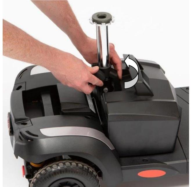
Place the battery pack in to the void in the scooter and ensure it sits flush. Press lightly on the top of the battery pack to ensure the battery pack is fully installed.
