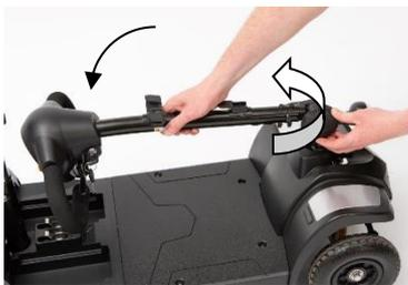
5. Turn the tiller knob anti-clockwise to loosen tiller. Lower the tiller and then turn the tiller knob clockwise to secure.
