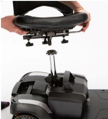
1. Push the Seat Rotate Lever whilst pulling up on the seat to remove.
