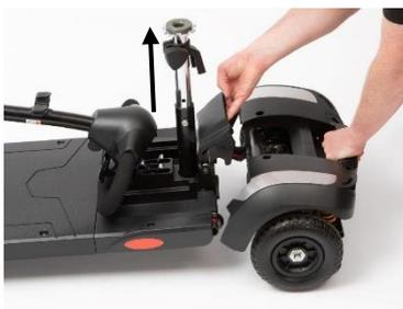
7. Pull up on the Connecting Handle to split the two halves of the base, whilst pushing on the rear of the scooter.
