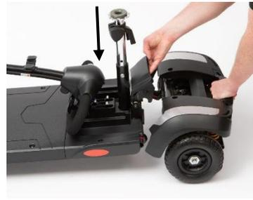
1. Line up the two sections of base. Lift up the handle and use the handle to slowly lower the two parts so they lock together, lining up the red markers.
