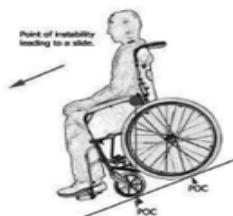
Figure 4 Beginning of instability (slope too steep)
