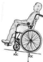
Figure 5 Stable on slope
