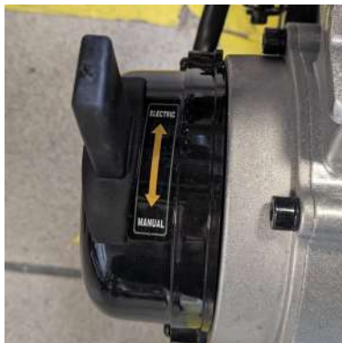
Figure 1 – Electric / Manual mode switch
